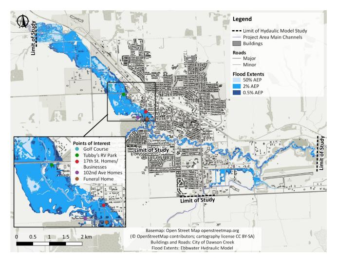
**Flood Hazard** maps are used to represent the total water depth, extents, and velocity. The map above shows the differences in flood extents between very small, moderately large, and very large (50%, 2%, and 0.5% AEP) floods. The darker areas are flooded under larger events; the map includes points of interest that were identified by Dawson Creek residents. The other flood maps can be accessed in the Flood Hazard Map Atlas.
